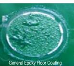
Condition after immersion for 24 hours in 20~30 % acid solution
